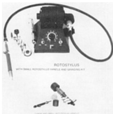
Fig. 4 Rotostylus. Courtesy of SIFCO Selective Plating
