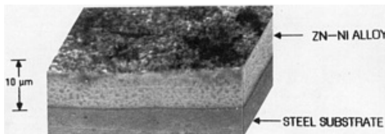
Fig. 3 Surface morphology and microstructure of zinc-nickel alloy coated sheet. Scanning electron microscope section. Source: Ref 11
